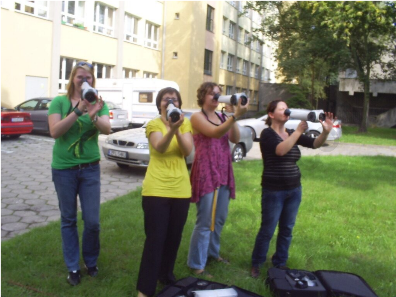
Nasal Ranger, an Olfactometer, in use
